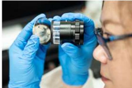
Check condition of ICP-MS Interface Cones
